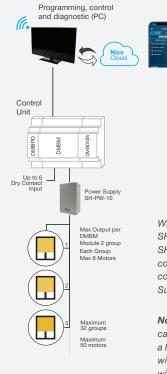
When paired, a SH-CT-50 and a SH-PW-10 provide a complete power and control solution for Sun Shades.
