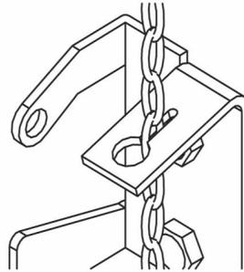
2. **If operator is supplied with optional floor level disconnect lever:** Pull disconnect lever downwards and lock in place by bending lever around bracket lip as shown.
