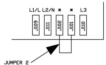
**WARNING:** When replacing the logic board in a single-phase operator. Make sure that Jumper 2 is installed properly before operating the door. Failure to do this will damage the logic board.
