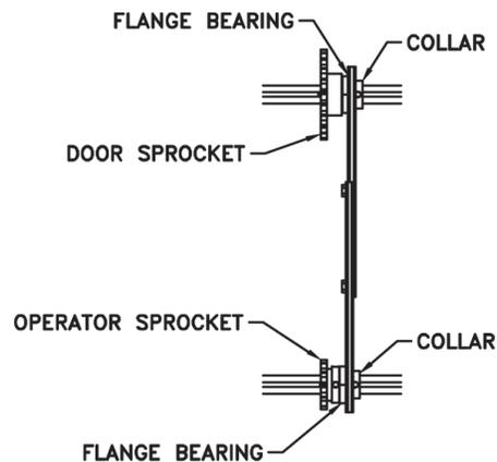
7. Install drive chain over sprockets, cut to a suitable length and connect with connecting link.
