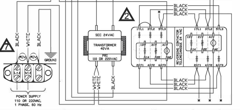
**1-PHASE WIRING DIAGRAM 110/220V**
