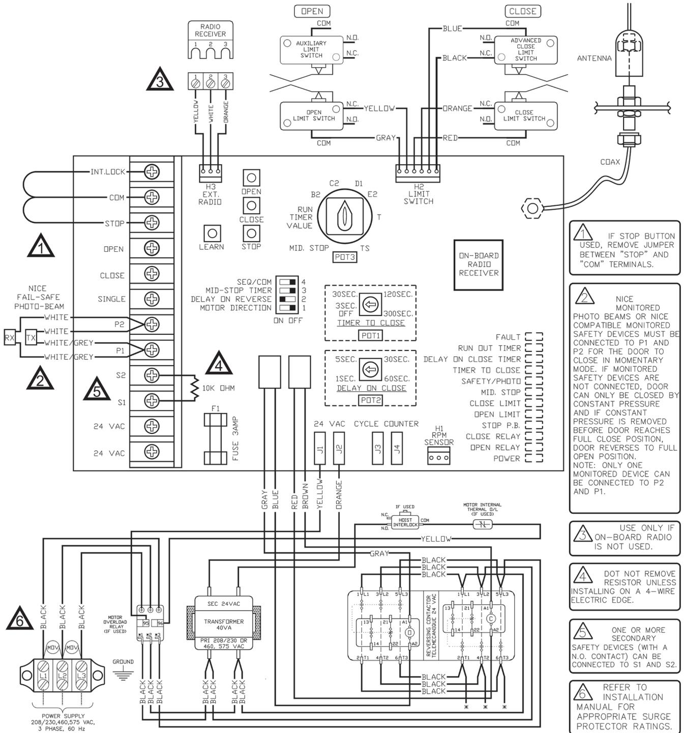
**1** IF STOP BUTTON USED, REMOVE JUMPER BETWEEN "STOP" AND "COM" TERMINALS.
