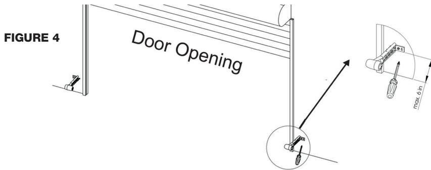
3. Plug sensors into flexible adapters as shown in Figure 5. Please note that the 2 brackets are not identical. The receiver (Rx) must be installed into the receiver adapter and the transmitter (Tx) must be installed into the transmitter adapter (Figure 6).
