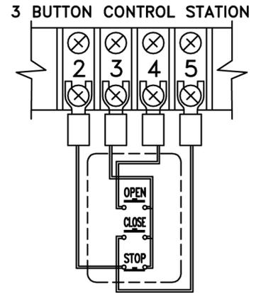
**CONTROL WIRING:** Use 7/8" (2.22 cm) diameter holes for all control wiring.
