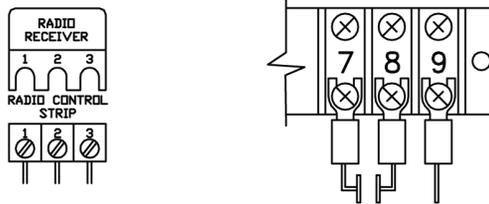
4. **Single button open/close device: Wire to terminals 7 and 8 on control terminal strip.**
