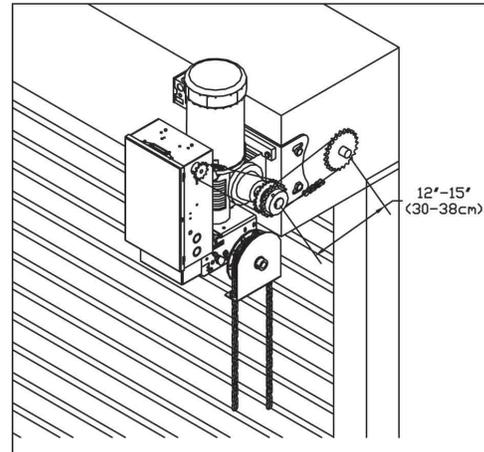
4. Mount the operator to the wall, hood or bench with 3/8" bolts, nuts and washers provided or with lag bolts and shields if installation requires it. Make sure that operator is secured but do not tighten bolts.
