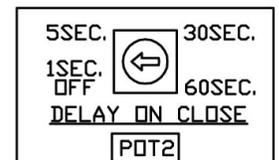
**NOTE:** In TS mode, the “Delay on close” timer starts only once the “Timer to close” has finished counting. Unless a delay on close is required this dial should be rotated to the OFF position. If left in any other position but OFF, activation of close button will delay to POT2 amount of time.
