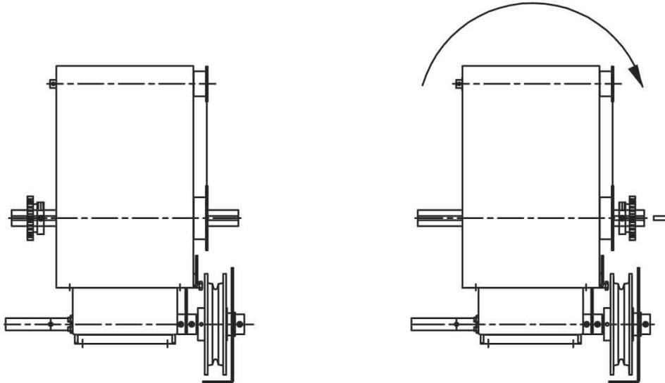
For both the PRO-GH and PRO-GHC operators the handing of the operator should be stated at time of order. Depending on installation, if handing of chain hoist is not correct the hand chain may hang in door opening. If this is the case, swing chain off to the side and hook it over the top of the door jamb. If desired, the pocket wheel, chain guard and hand chain may be removed on site and installed on opposite side of universal disconnect shaft as shown below.
