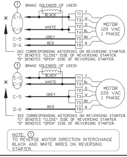
NOTE: ① TO REVERSE MOTOR DIRECTION INTERCHANGE BLACK AND WHITE WIRES ON REVERSING STARTER.
