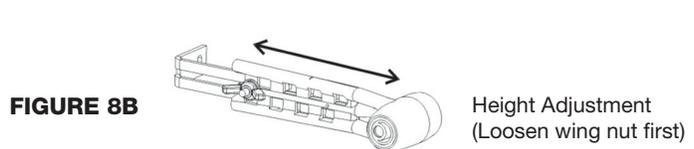
6. Utilize LEDs on photocells for alignment and trouble shooting. Make sure to tighten screws and wing nuts after photocells are aligned.
