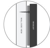
4. Slide and lock back keyhole slot over exposed screw and position unit vertically.
