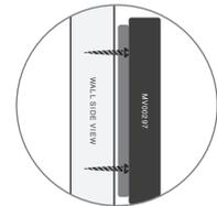
6. Insert bottom screw and tighten and re-install battery door.
