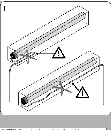
**CAUTION!** - <u>The smaller cables must be handled carefully</u> because they contain very thin wires that could be damaged.
